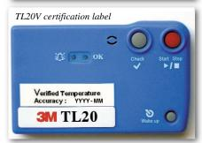
PC software is user-friendly for customization, functionality, and reporting. View time and temperature data as a graph or in a spreadsheet. Temperature monitor connects to software with a USB cable.
